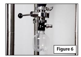
Tighten the collection bottle to the harvester body and remove the gas ball lock.
