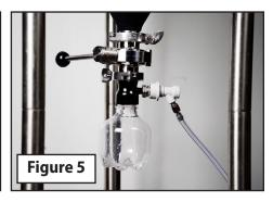
Attach the gas ball lock and introduce CO2 into the collection bottle. Five seconds of purging at 10psi is sufficient.
