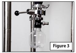
Install the Yeast Harvester as shown in figure 3 with a 1.5" tri-clamp and gasket.
