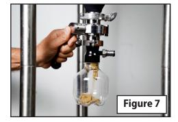
Slowly open the valve to allow the yeast into the bottle. After the yeast has been harvested, close the valve and slowly unscrew the bottle to gently relieve pressure.
