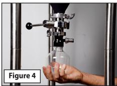
Slowly loosen the collection bottle to allow CO2 to release out of the top.
